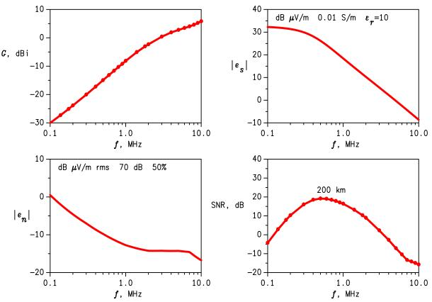
Figure 5. Factors contributing to the SNR of a ground-wave signal.
