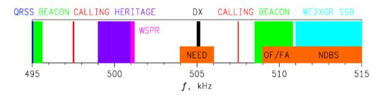
The segment of the band labeled "Heritage" refers to spectrum used by commercial services such as maritime stations (although many have abandoned 500 KHz to use satellite communications).
