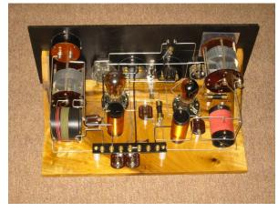
**▲** Behind the MOPA panel. Ladder line feeds a 160 meter dipole as the hat of Brian's Marconi T transmitting antenna.
