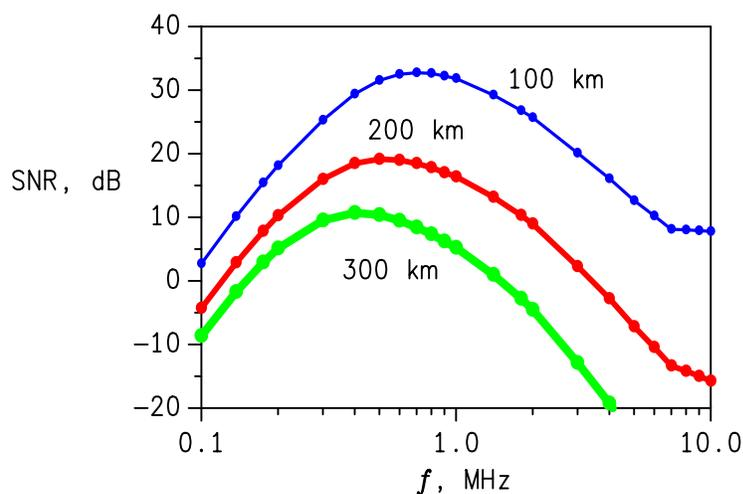
Figure 2. Ground-wave SNR as a function of frequency for typical amateur use.
